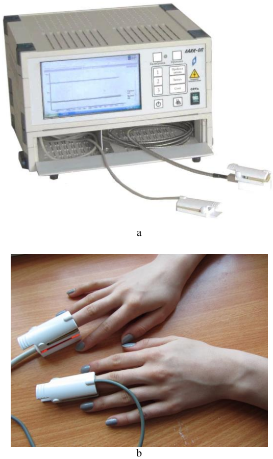
Fig. 1. The «LAKK-OP» laser analyzer of blood microcirculation used by general practitioners (a) and position of the optical sensors on the fingers of volunteer during the research (b)
